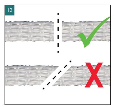
NOTE: Cut the Tube-Tape at right angles to its length to minimise the generation of loose fibres. Take care to remove any loose fibres that are created.
